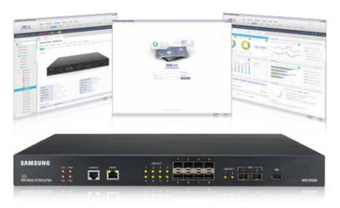
The WEC8500 is a high performance WLAN controller that is able to simultaneously manage up to 500 access points and operates at 20Gbps, offering a fast and reliable network.
